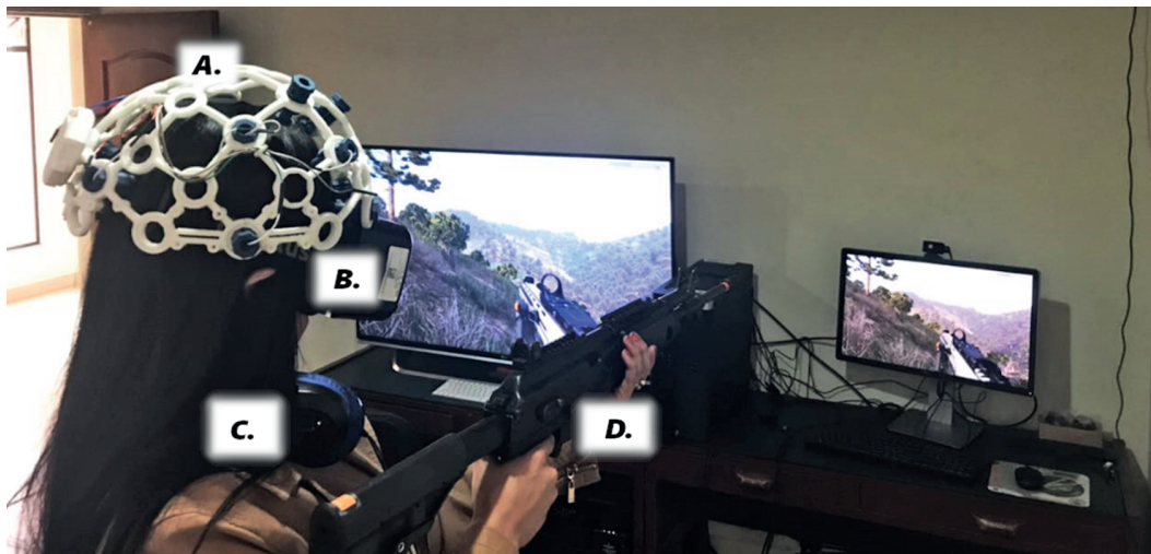
Figure 3. A standard virtual reality set-up implemented at the "Centro de Investigación y Desarrollo en Simulación – CIDSi", composed by: A.) electroencephalogram headset [Open bci], B.) head mounted display [oculus Rift], C.) headphones, and D.) weapon adapted as a peripheral input, the vr environment projected on displays is provided by the platform Virtual Battle Space.
